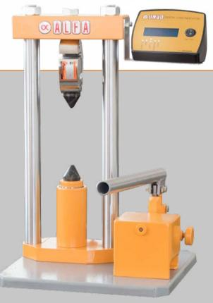
Point Load with Load Cell and Digital Readout Unit (RM-120/LC)
