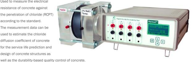
Perma2™ is electrically certified for rapid chloride penetrability test in concrete laboratories and its measuring cell sizes are . according to the ASTM and AASHTO specifications. Equipped with a verification kit, Perma2™ is an accurate test device for concrete labs.
